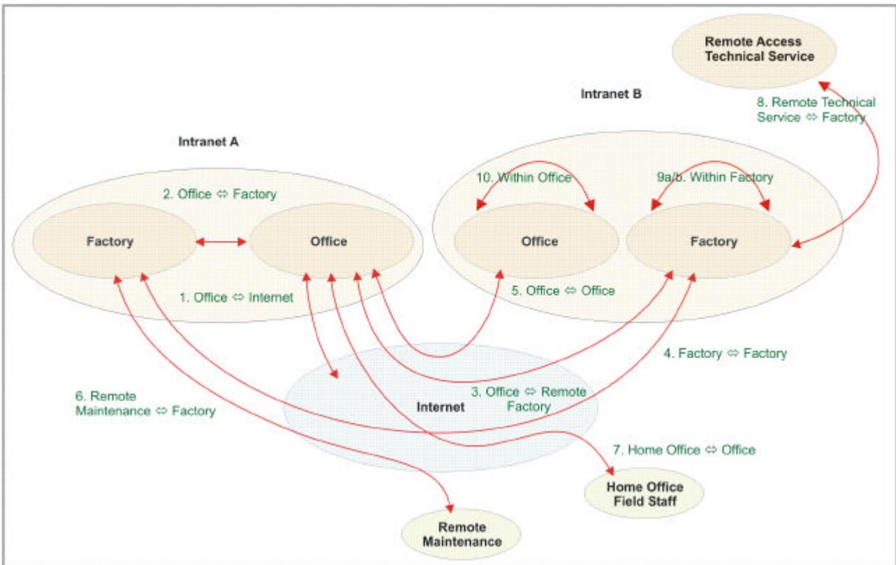
**Figure 5: Communication relations of a company network**
