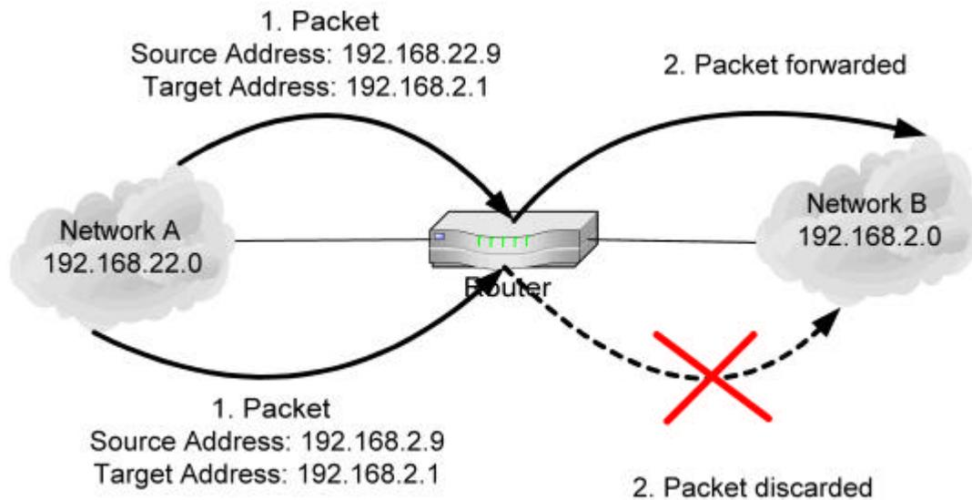
**Figure 15: Filtering packets with invalid addresses**
