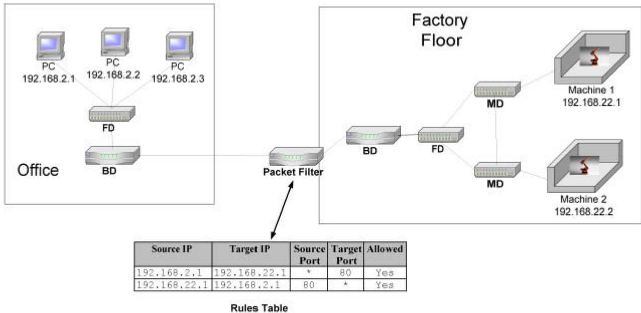
**Figure 11: Packet Filter Example**
