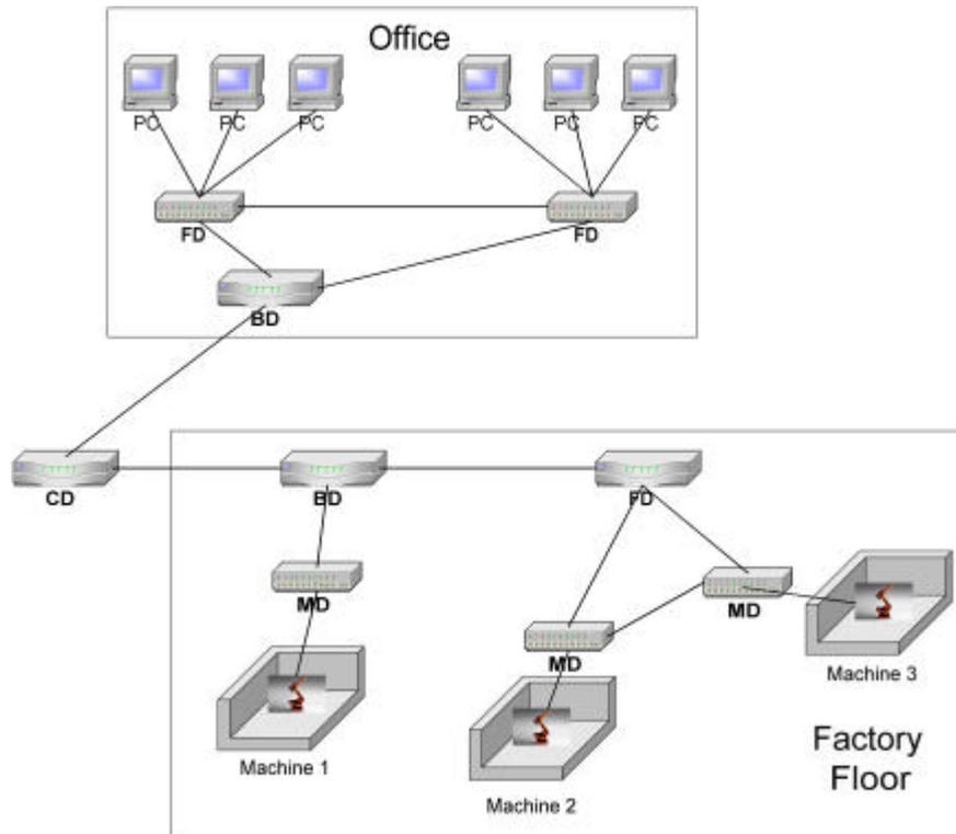
**Figure 7: Example of a network topology according IAONA**
