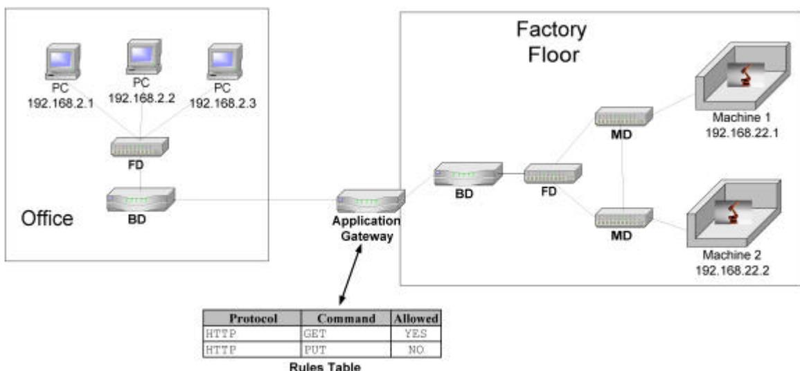
Figure 13: Usage of an Application Gateway
