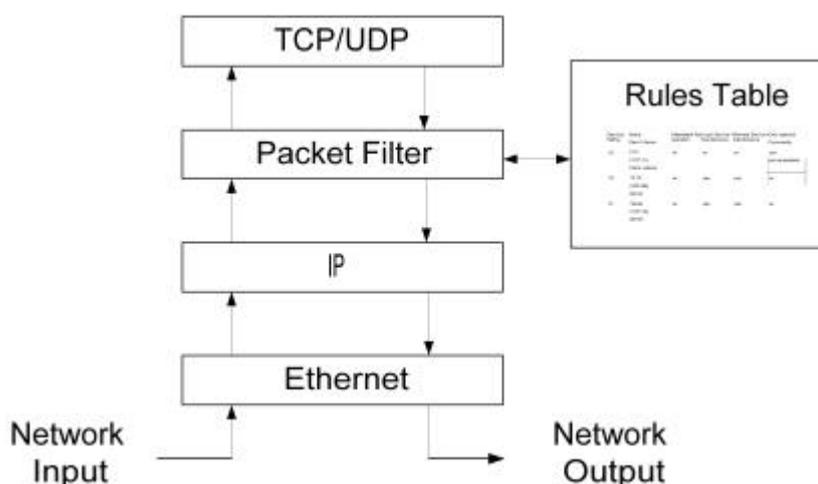
Figure 10: Concept of a Packet Filter
