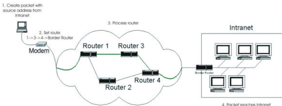
Figure 3: Source Routing
